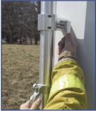
Kwik-Release cam latch securely holds pole to truck.
